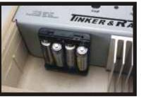
The CI-50 uses AA batteries. Easy to find and easy to replace. The AA batteries in the CI-50 will keep it operating for more than 80 hours.
