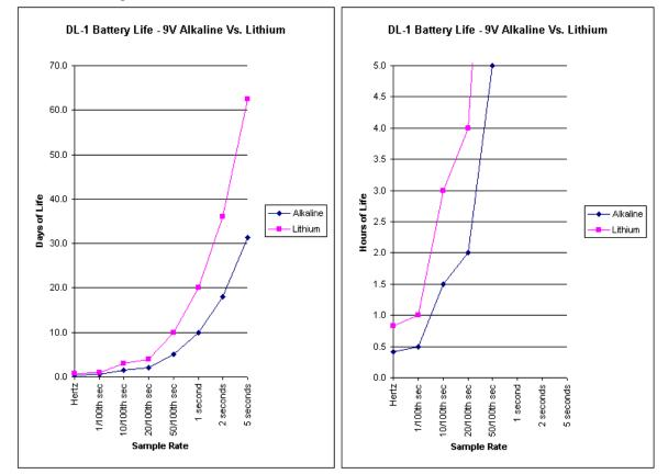
The Sample Interval directly affects battery life; each sample recorded consumes a fixed amount of power. To be sure a logging sequence will run to completion before battery power is expired, find the desired logging sequence Total Run Time on the "Battery Life (Days of Life)" axis on this chart. A horizontal line drawn through this point will intersect the curves for various Sample Intervals, indicating valid combinations of the sampling and flash
