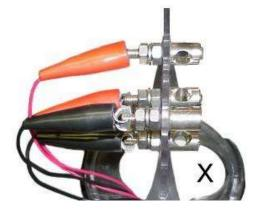
Connect the Data Logger in the field using the included cable with four pairs of clamps. The clamps make it easy to connect to test stations, like the connection at left between the DL-1 Data Logger and the Tinker & Rasor CP Test Station Model T-3.
