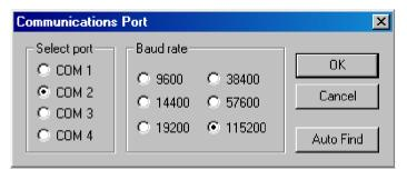
From the Communication pull-down menu, select Setup to setup or change the communications port selection for the PC. At left is the dialog box that appears. Select the correct COM port or use Auto Find. Auto Find will find the correct port if the logging unit is in the "Off" mode, and is connected to an available COM port on your computer. This will only need to be done once, unless the PC's hardware is changed or a different PC is used.
