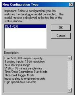
Before recording information with the logging unit, you must first configure it. This is done by creating a configuration 'document' and then sending it to the logging unit. Configuration documents can be created once and saved to disk for reuse in future data collection tasks.
