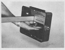
Fig. 2 — MOUNT TRANSMITTER ON HANDLE, making sure handle is fully inserted in mounting hole.
