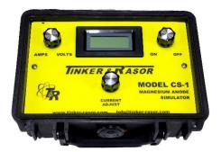
Control panel description: On / OFF – Used to turn the CS-1 current and panel meter on and off.
