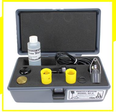
The Model SC-4 Sliver-Silver/Chloride kit come complete with everything necessary to conduct field tests both ON SHORE and OFF SHORE.
