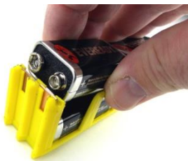
Figure 14 – slide battery in observing polarity
