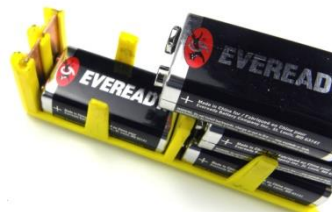
Figure 7 – all batteries must be installed the same way
